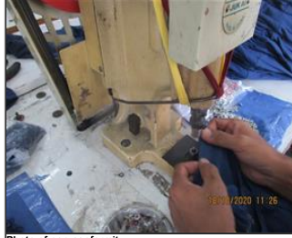
Photo of non-conformity NC 7.17-Finger safety guard was found non functional at snap button machine.JPG
