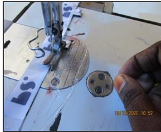
Photo of non-conformity NC 7.17-Needle guard found inappropriate position in sewing section.JPG
